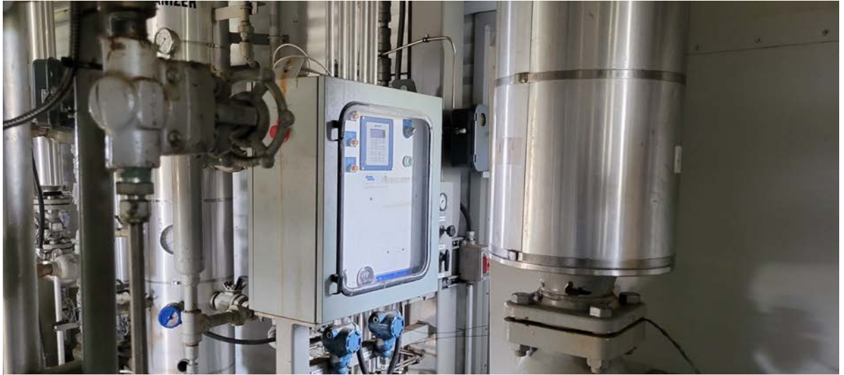
Altronic DE-2500 control panel (bottom picture, and all vessels U-Stamped and available registration for all other Canadian provinces)
